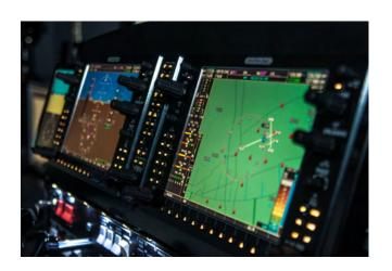
This proven, high fidelity G1000 simulation software provides about 85% of real G1000 functionality—far and away more than other simulations. Here are some of the features that separate the PI-1000 from its competitors:
